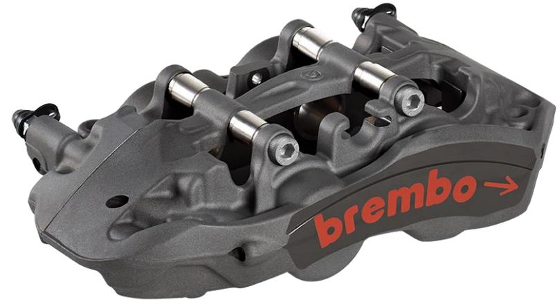
4 pistons, 28/30 – 36/42 mm (1.10/1.18" – 1.41/1.65"), suitable for disc diameter 315 – 330mm (12.40" – 12.99") and disc thickness 28mm (1.10")
