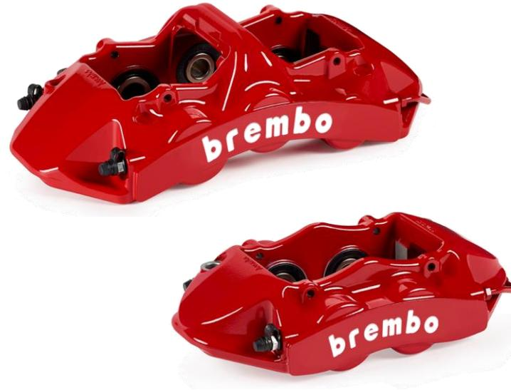
Monobloc calipers that are specifically designed to offer high-level performance both in normal road use as well as for the demanding days on the track, with a unique style given by Brembo's exclusive geometries and design.
