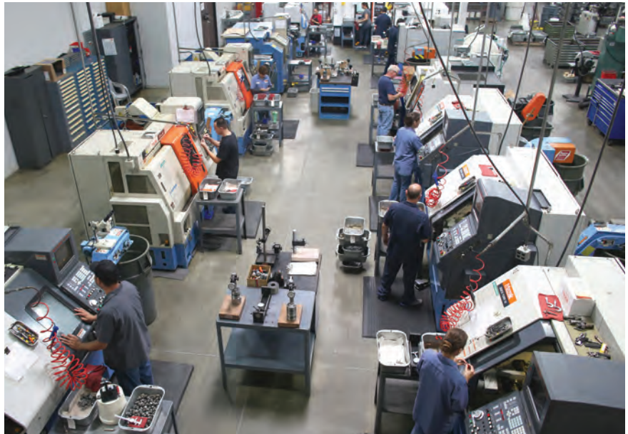
A bank of CNC machining centers are employed at ARP to perform specialty operations.
